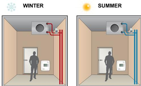
In 4-pipe installations, there are two separate water systems for heating and cooling with separate valves. The controller uses two outputs for control of heating and cooling in sequence with two thermal actuators.
