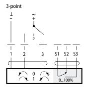
Auxiliary switch Connected with conductors S1, S2 and S3 (only model RDAB20-24S)
